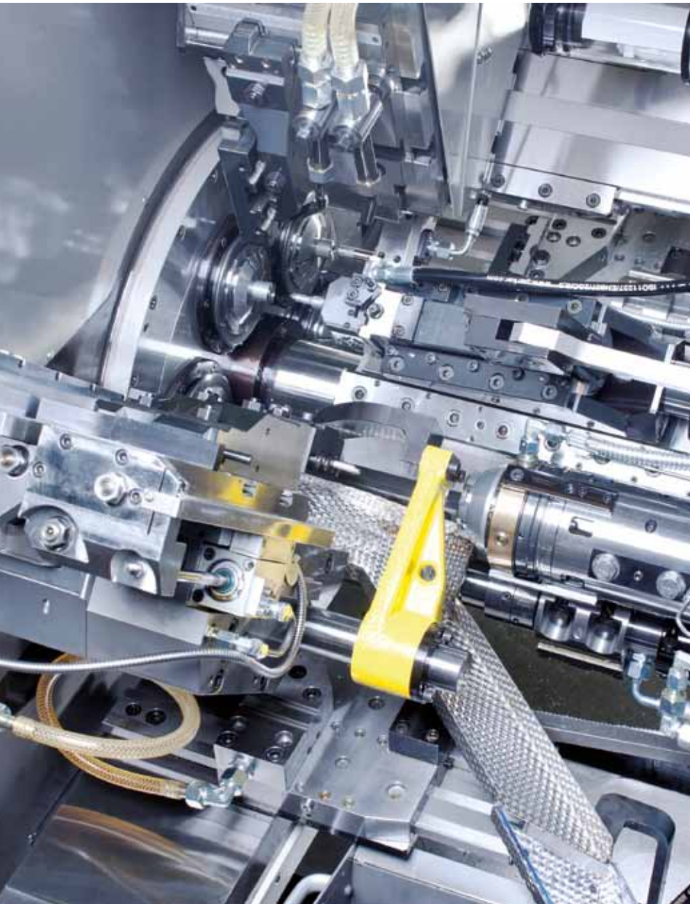
Material removal area of a six-spindle automatic of the PC series
